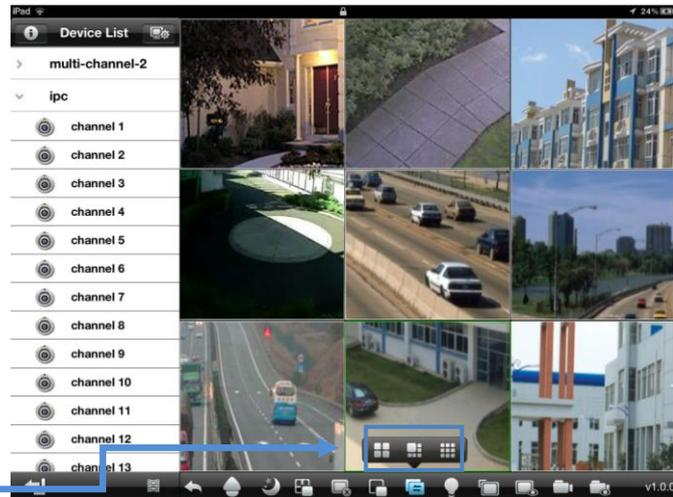
Touch a channel on the screen and drag it to the channel position to rearrange your viewing window.
